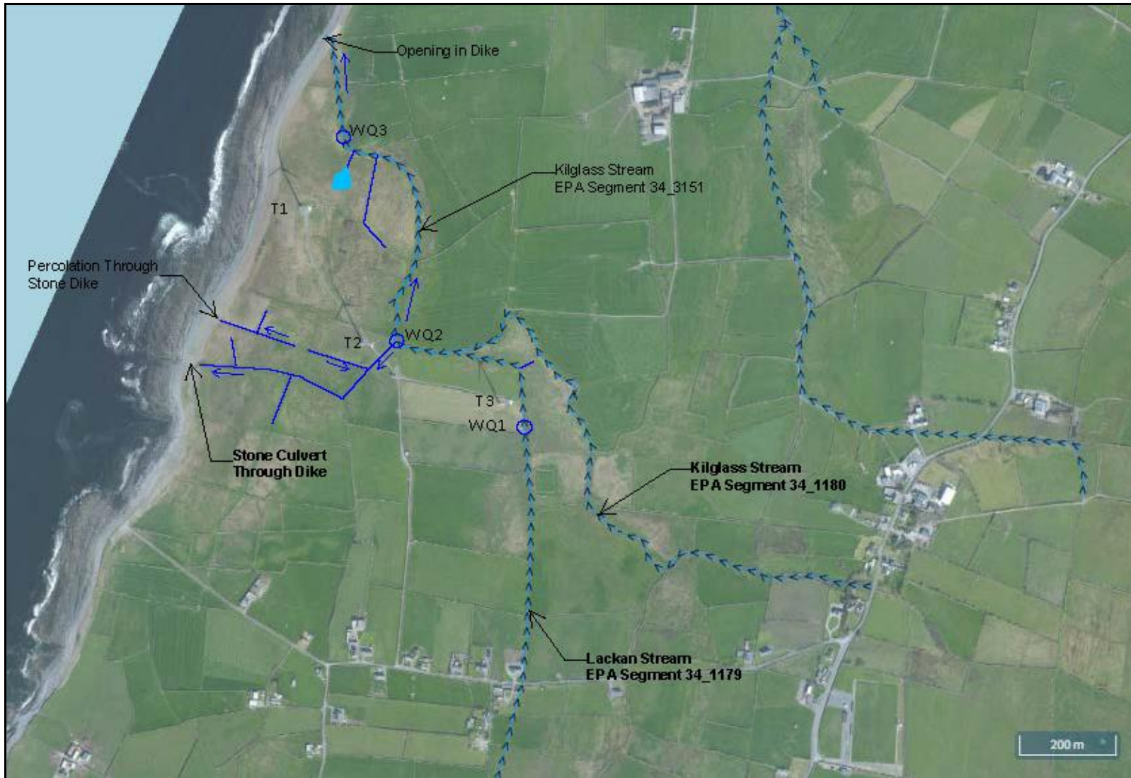
Figure 7-1: Site Drainage Details
